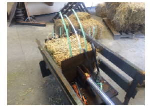
Double compressing bales to density of 25 lb/sq ft.
