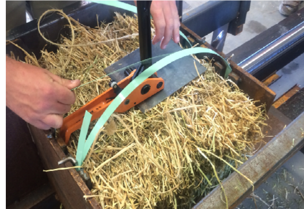
Double compressing bales to density of 25 lb/sq ft.
